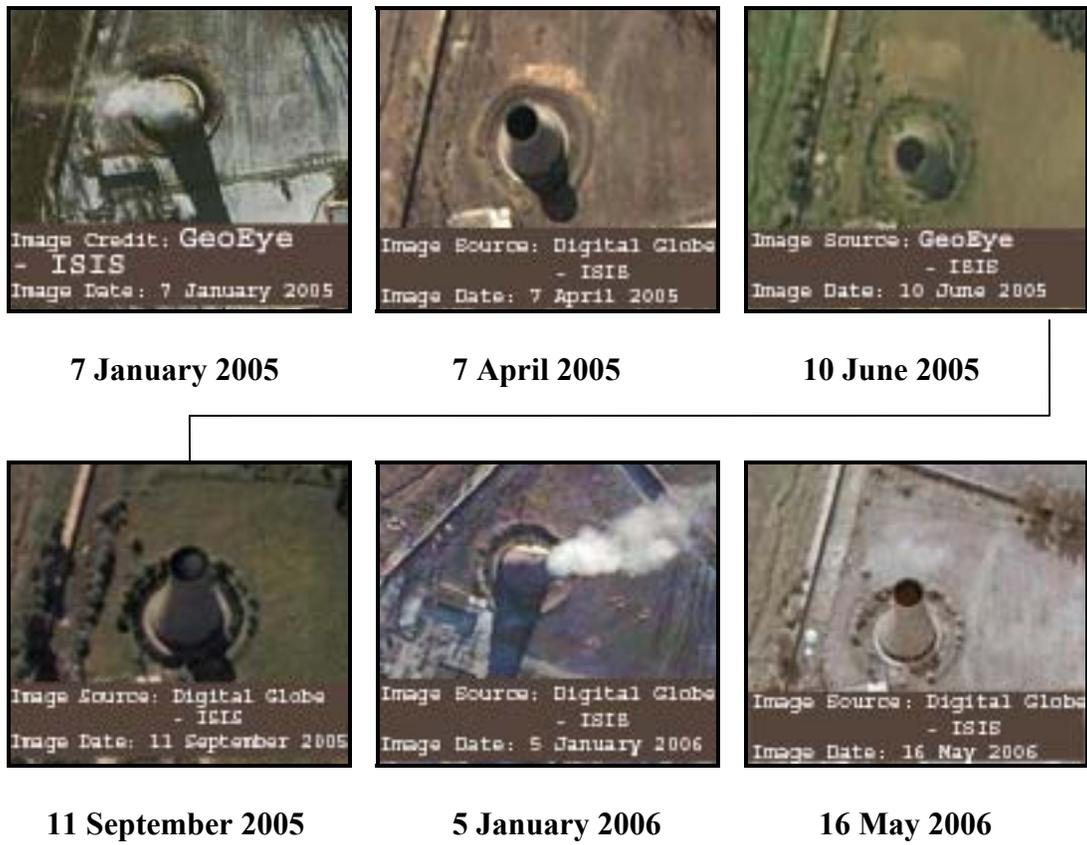
**A composite series of images showing the cooling tower at the 5 MWe reactor. A plume is visible in January 2005 and is not visible in the images from April and June 2005. A plume is visible in September 2005 and January 2006. In the most recent image, from May 16, 2006, a plume is not visible above the cooling tower.**
